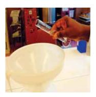
3. Glycerol is added using a measuring cylinder. As glycerol is very viscous and sticks to the wall of the measuring cylinder, it should be rinsed with some sterile distilled or cold boiled water and then emptied into the bottle/tank.
