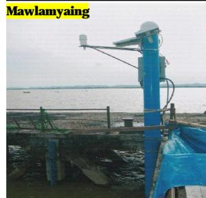
🚧 Sea Level Gauge (for Tsunami Warning) installed on 2006 (donated by UNESCO-IOC)
