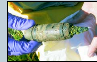
A full DU round found on a surface (penetrator already corroded)
