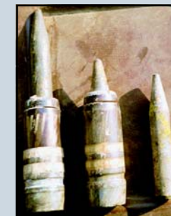
30mm DU munition: jacket and penetrator
