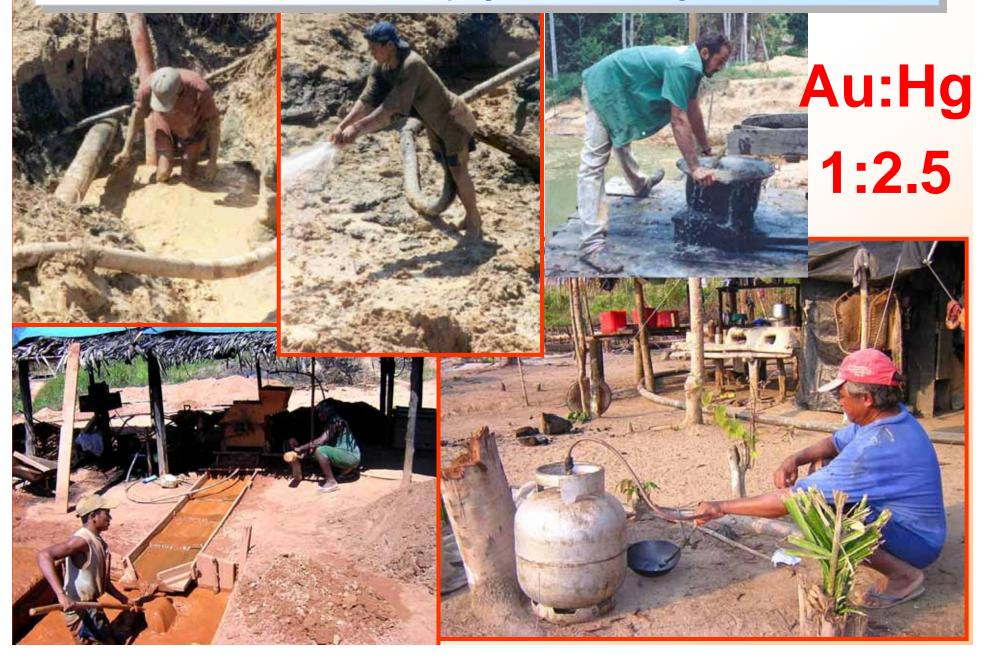
SGM as Hg source to the environment: waste discharge: tailing ponds or directly in waterbodies Primary gold ore: Hg associated to Cyanide Amalgam burning: in the field or gold shops to the atmosphere
