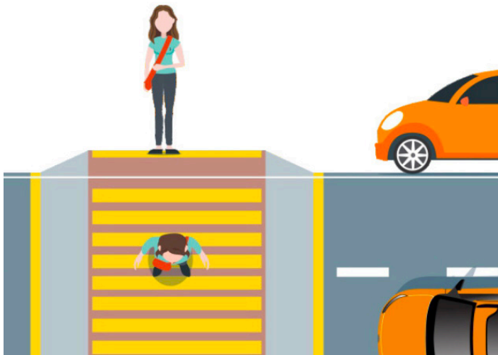
The Guideline recommends raised pedestrian crossings
